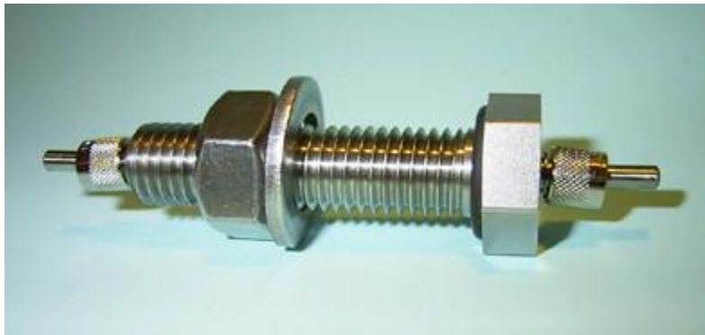
The FC-VFT vacuum feedthroughs are designed for use of fiber optics in vacuum chambers, such as for plasma monitoring. The vacuum feedthrough consists of an M12 housing with Viton® O-ring and 2 SMA fiber optic interconnects to allow easily coupling to fiber optic cables and probes. The vacuum feedthrough can be delivered for all fiber diameters, such as 50 µm up to 1000 µm for UV/VIS as well as for VIS/NIR. (This is a product of Avantes, Inc., 9769 W. 119th Dr., STE 4, Broomfield, CO 80021. http://www.avantes.com/ )
